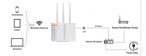
Passive PoE – The KP322 is able to be powered using an Ethernet cable up to 30 meters. Allow you to place the device more flexible and effortless.
