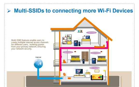
**Multi-SSID** –enables users to configure up to 8 separate SSIDs ( $2.4 \, \text{GHz} \times 4$  and  $5 \, \text{GHz} \times 4$ ) in order to group and manage users according to your requirements. In addition, each SSID can be assigned a different VLAN ID, so users with multiple VLANs can manage the network access level of each SSID - ensuring security and protecting confidential or critical network resources, ensuring protecting confidential or critical network resources.
